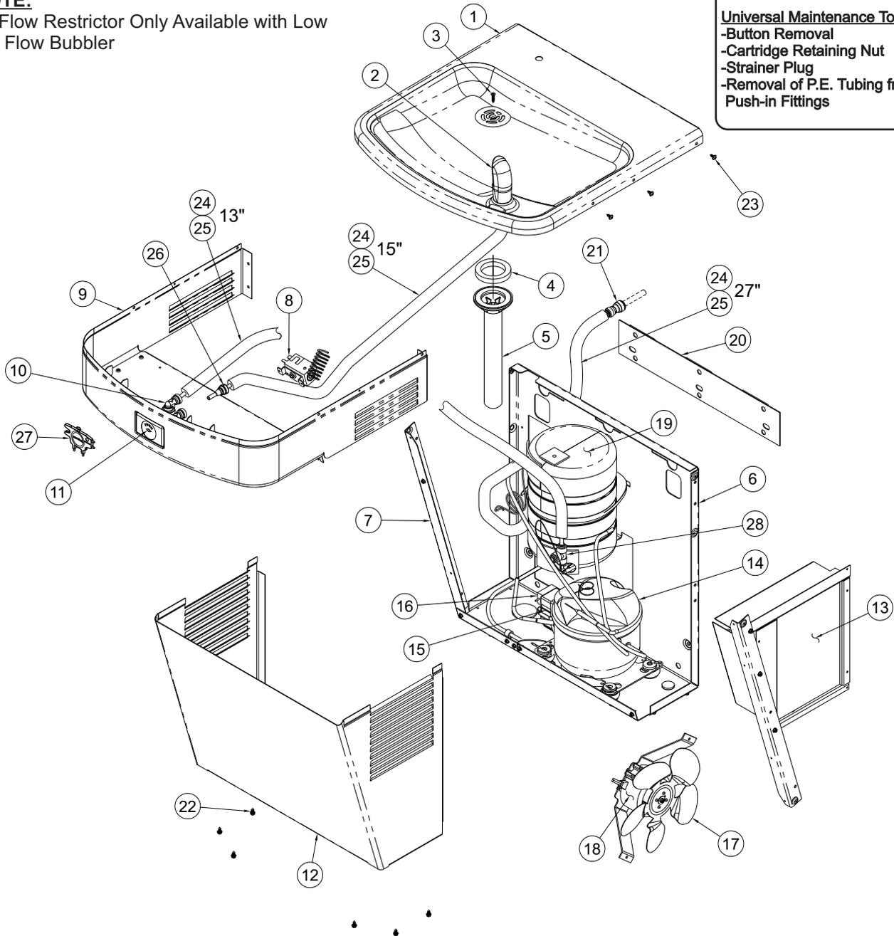
Standard A171.8-UG-BFxS series refrigerated ADA Water Cooler shown. All 1/4" O.D. Plastic Tubing (24) must be insulated with (25) foam insulation.
